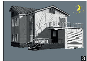
3 After hold time, the sensor switches off the lamp when no motion is detected.
